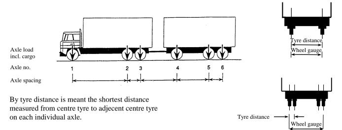
Wheel gauge width is measured from centre tyre to centre tyre.
