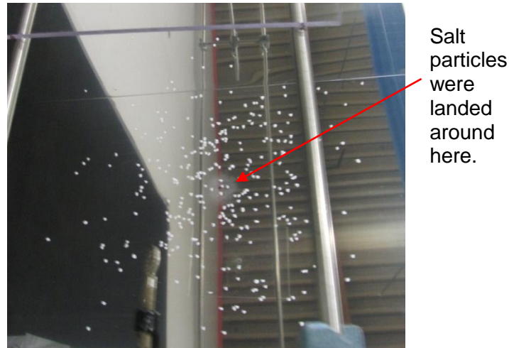
Figure 6: Distribution of salt particles after bouncing on a horizontal stainless steel plate.
